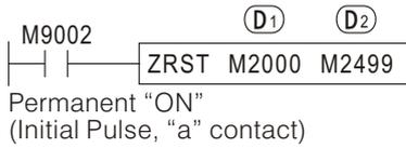
D1: the device starting the Range Reset.
